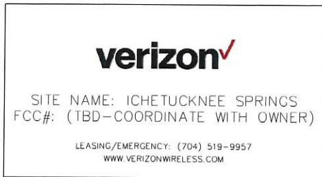
① VERIZON AND FCC REGISTRATION SIGN SIZE: 12"X 24" (0.063" ALUMINUM) (TO BE MOUNTED ON GATE)
