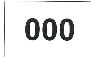
④ E911 STREET # LETTERS MUST BE A MINIMUM 5" TALL (TO BE MOUNTED ON THE FENCE FACING THE ACCESS DRIVE)
